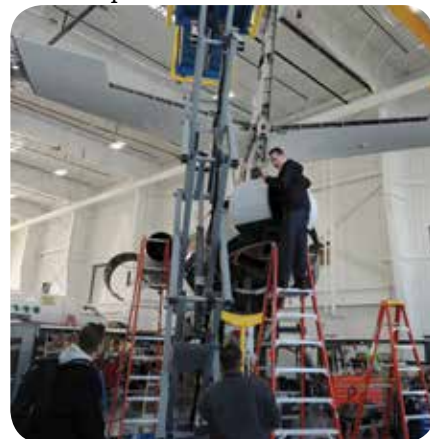
Dassault Falcon Undergoing 3 Week “C” Inspection
