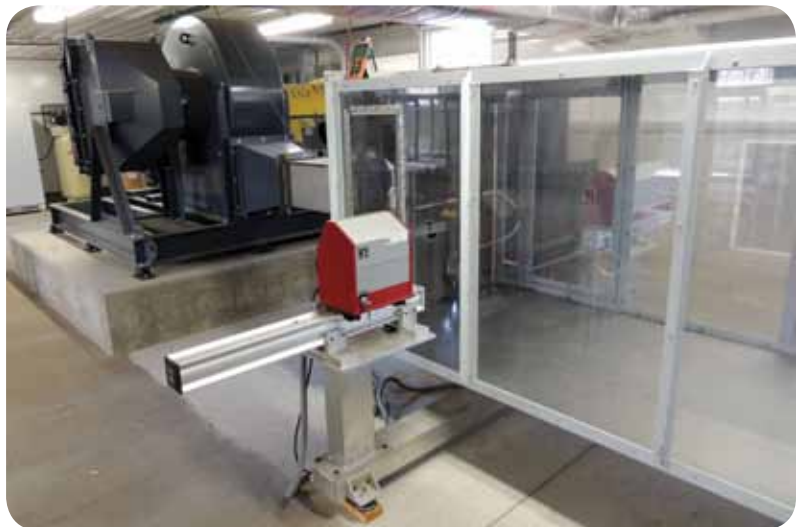
High-speed wind tunnel powered by 200 hp electric motor
