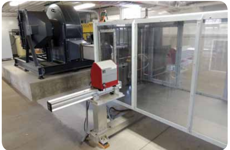
High-speed wind tunnel powered by 200 hp electric motor
