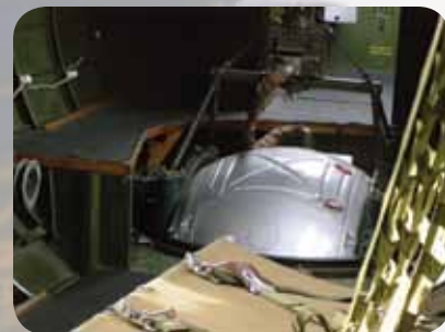
The Ball Turret is The Shiny Dome in the Floor
